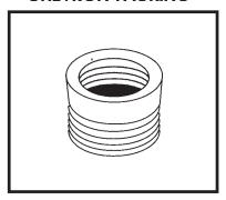
The ChemValve® Model 790EB-300 high performance lined plug valve has adjustable chevron TFM packing like a globe valve. The six ring set is much more substantial than the thin diaphragms used in other lined plug valve designs. If process pressure leaks into one of the packing rings, it will mechanically spread the ring sealing off the leak. This means there is little chance of either corrosive stem leakage onto the bonnet of the valve or fugitive emissions to the atmosphere.
